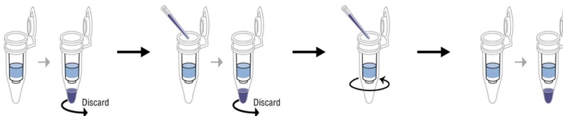
1. Add detergent removal resin (25-200 $\mu$ L) into Micro Spin Column and centrifuge for 1 minute at 1500 x *g* to remove the storage buffer. Discard the flow-through.
