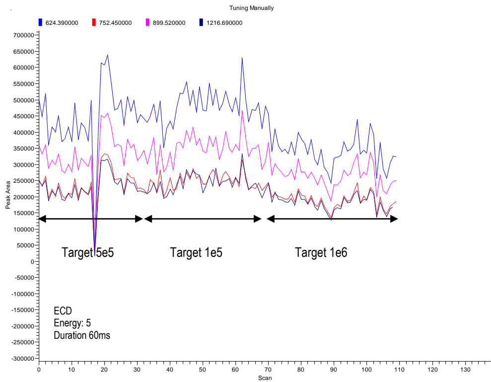
Substance-P ECD fragments at different target values, with fixed energy and duration
