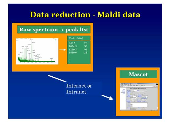
This is the simplest example of data reduction. This is a typical maldi spectrum which contains about 50,000 data points. We need to reduce this to somewhere between about 30 and 150 peaks. Unfortunately, this is not as trivial as it seems, and we are still seeing people perform this process manually for some spectra.
