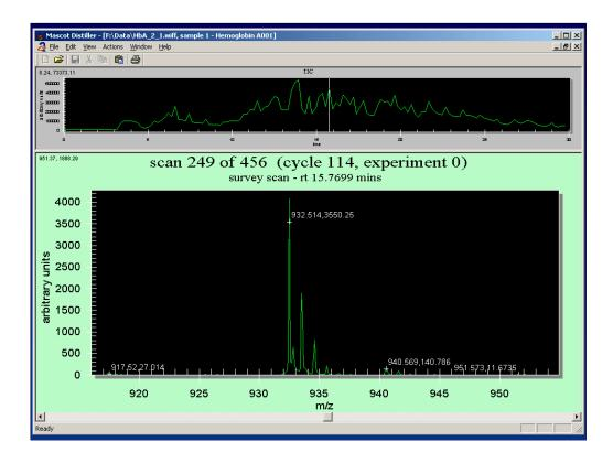
... we can see a nice looking isotopic cluster that any peak detection software would detect - although some of the poorer algorithms will unfortunately detect and label the carbon 13 and carbon 14 peaks as well. I would just like you to note that the intensity of this peak is about 4000.
