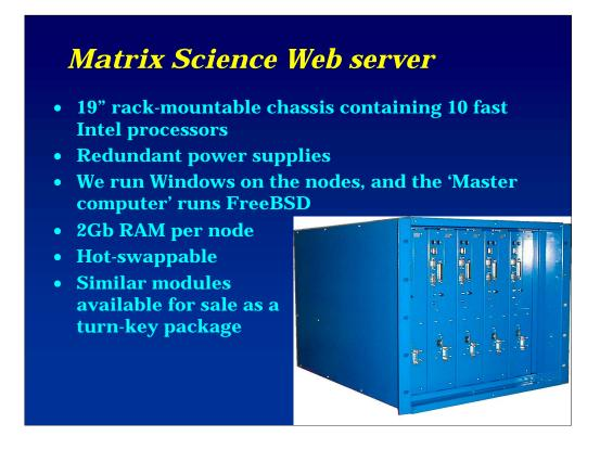
Alternatively, we can supply a complete turn-key solution based on rack mounted, high-reliability PC hardware. Our web server uses this hardware
