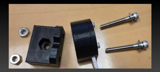
Socket Head Screw, 8-32 Thread Size, 1-1/2" Long, Partially Threaded (92196A203 McMaster-Carr)
